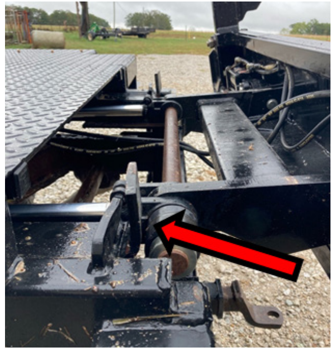
RESULT OF INCORRECT SPIKE POSITION
