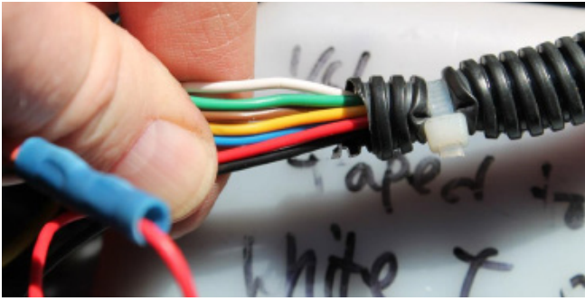
Blue wire attaches to top outside manifold coil. (butt splice with blue hand control wire)
