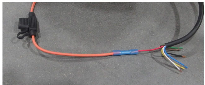
Red wire connects to the orange fuse wire.
